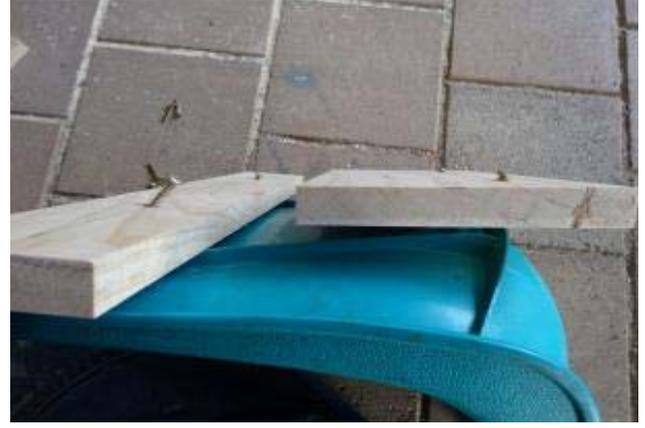
here is a pic showing the angle of the screws through the timber to the seat
