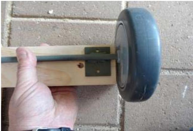
Line up the Front Axle as pictured so the axle is offset forward so as to miss the center bolt and rope holes and Screw it down
