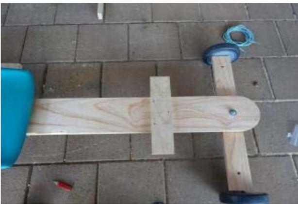
Position the Foot Rest (#7) timber in position this is all dependant on the childs most seating position and screw it down with 3 counter sunk screws once centered
