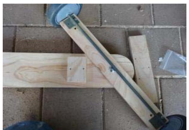
Here is the steering block in use it limits the front steering rail from turning too far and leading to possible mishap
