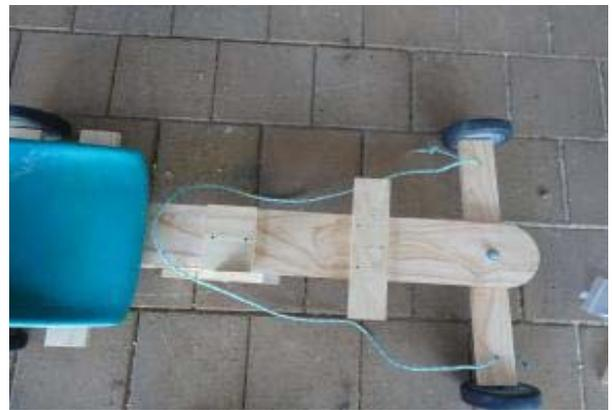
Here is the finished rope position, please note rope steering can not be used in the Billy Cart event, a steel or similar steering hoop must be used for safety reasons (better Control)
