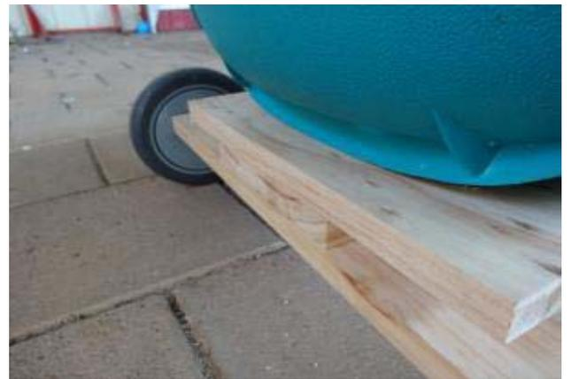
Line the back of the Rear set mount timber up with the back of the main strut and square it up and screw it down with the counter sunk screws (2 per seat rail from under neath)
