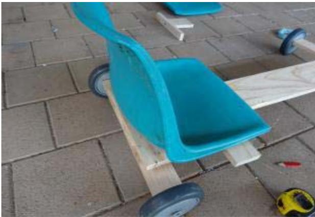
With the seat timbers and seat loosly mounted Position it on the main Strut at the back end
