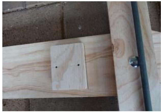
Position the Steering Stop Block on the under Side of the Main Strut, you will see a pencil line as a reference, then center the block
