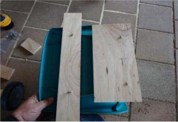
Position the Seat Mount Timbers on the Plastic Chair as shown, loosley fit the screws to the timber (ensure the angled holes match)
